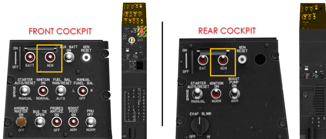
Figure 1-13 Generator Switch Location/s
